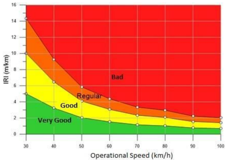
Figure 1: IRI vs. Operational Speed with Regions of Acceptability, from Abudinen et. al.
